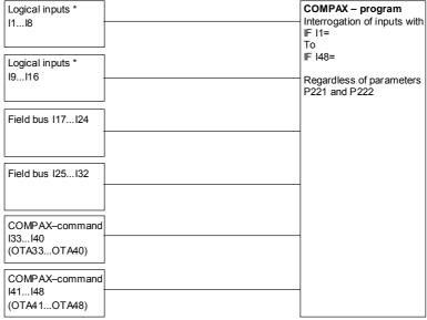
With P233=48 (or P234=48), virtual inputs I48 – I25 are written to the optimization display status S13 (S14). Meaning: I25 = bit 0 ... I48 = bit 23.
